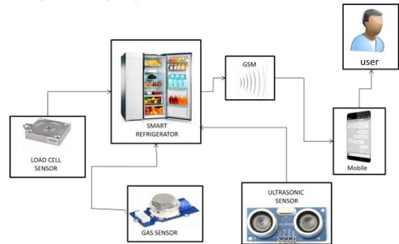
Fig 1.1 System Architecture for a design of smart refrigerator.
