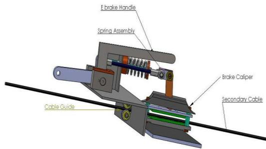
Figure 1. Models of the complete Braking System
