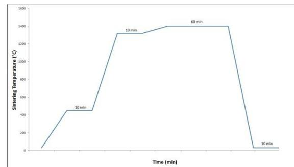
Fig. 2. Heating schedule used for the sintering process
