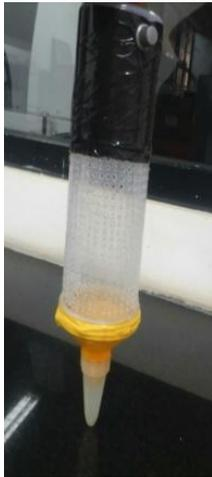
Fig. 2 Solar light glue Trap
