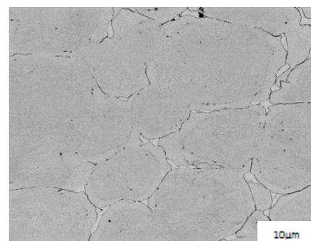
**Fig. 6: The microstructure of CoCrMo alloy after etching.**
