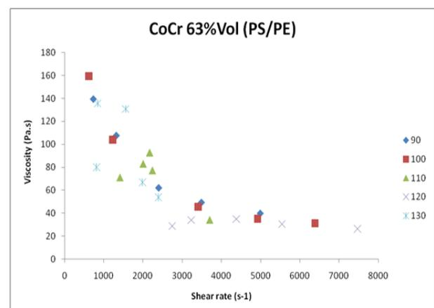
**Fig. 1:** The graph of viscosity versus shear rate for 63vol.% of powder loading formulations of PS and PE at different temperatures
