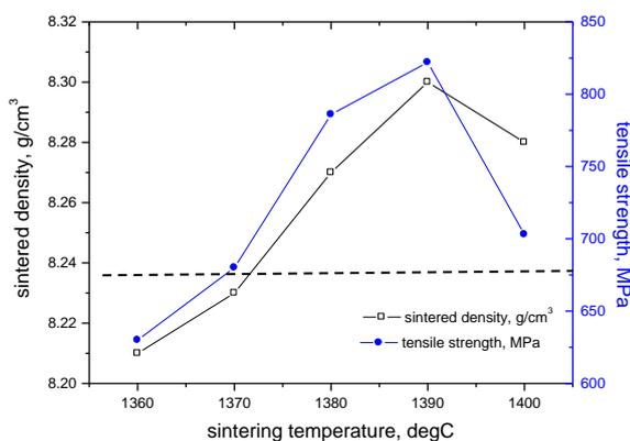
**Fig. 4: The effect of sintering temperature on sintered densities and ultimate tensile strength**
