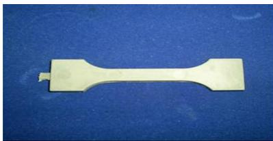
Fig. 2: The tensile shape of the injection moulded parts with a single gate, located at one end of the part
