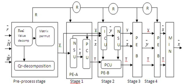
Fig.2 VLSI architecture of MIMO signal detector
