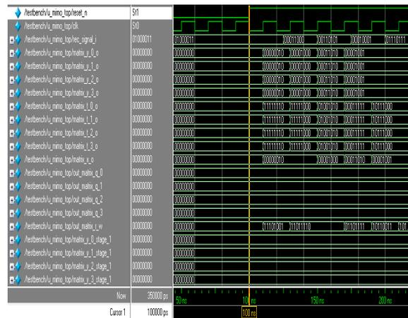
Fig.6 Output Waveform of MIMO detector
