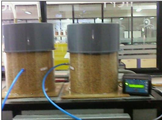
**Fig 1. Acrylic bin for CO<sub>2</sub> fumigation**
