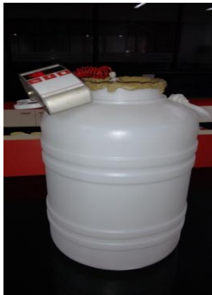
Fig 2. PVC bin for CO 2 fumigation
