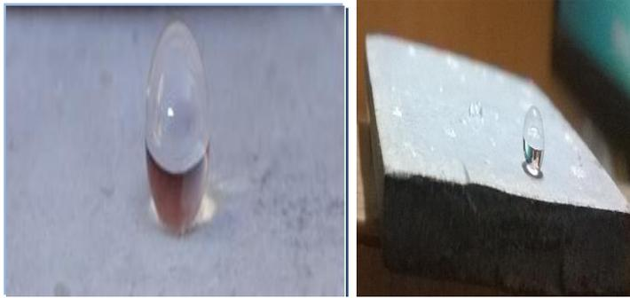
Figure 1. Digital photographs of one water droplet on surfaces of (a) Al6061, (b) etched Al6061, (c) superhydrophobic surface with various CA.
