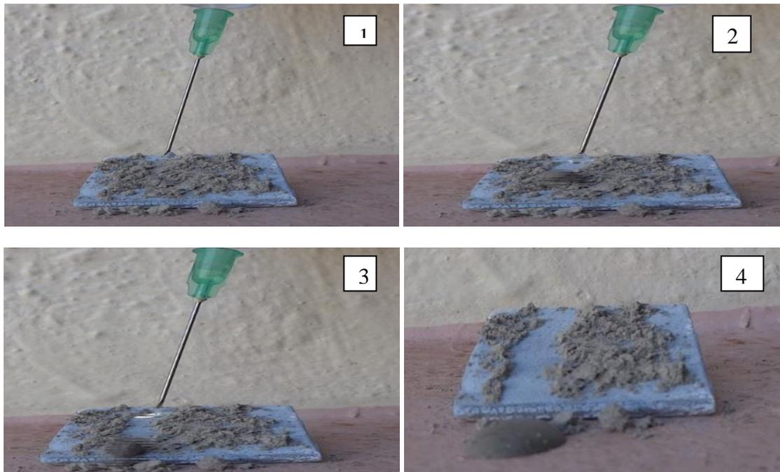
**Figure 3.** Self cleaning property showing dust particles cleaned at different stages
