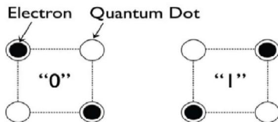
Figure 3: Four Dot QCA Cells [6]
