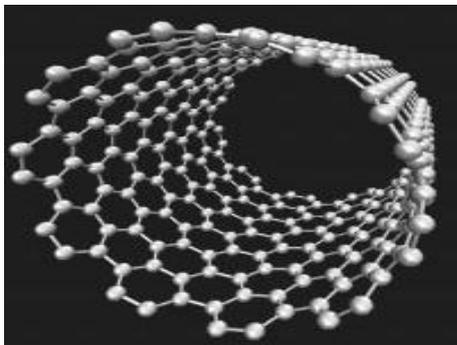
Figure 1: A single walled carbon nanotube [4]
