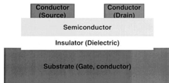
Figure 4: Typical structure of an Organic Field Effect Transistor [7]
