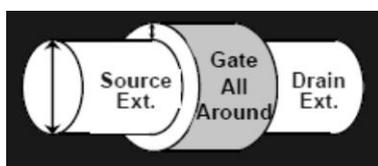
Figure 5: Silicon Nanowire Device Structure [9]
