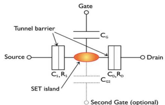
Figure 2: Schematic of basic Single electron transistor [2]
