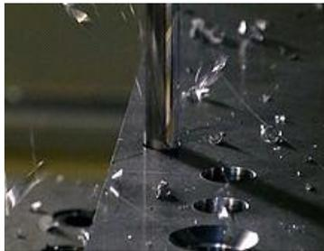
Drilling is a cutting process that uses a drill bit to cut or enlarge a hole of circular cross-section in solid materials. The drill bit is a rotary cutting tool, often multipoint. The bit is pressed against the work piece and rotated at rates from hundreds to thousands of revolutions per minute. This forces the cutting edge against the work piece, cutting off chips from what will become the hole being drilled. Exceptionally, specially-shaped bits can cut holes of non-circular cross-section.
