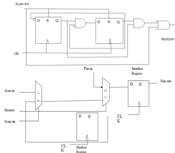
Fig. 1. DFT support for restore operations in LOC testing
