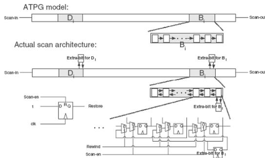
Fig. 2.ATPG model and actual scan architecture for low-power LOS testing
