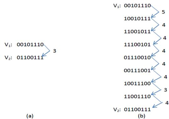
Fig. 5. (a). Transitions between 2 test vectors. (b). Unnecessary transitions in scan architecture
