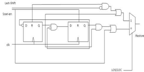
Fig. 3. Unified restore signal for mixed testing with LOC and LOS patterns
