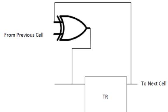
Fig. 6. Scan cell structure of the proposed architecture
