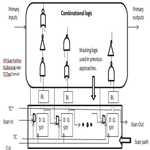
Fig. 4(a).Scan architecture with blocking circuitry
