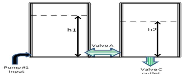
Fig.3: Schematic Layout Diagram of SISO Two-Tank Setup[8]
