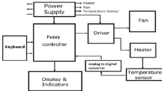
Fig .6: Block Diagram of Temperature Control System[13]
