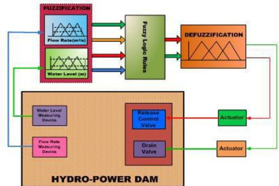
Fig.4: Block Diagram of Hydro-Electric Power Dam Fuzzy Control System [11]
