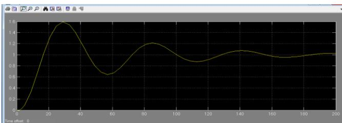
Fig.7 (a): Step Response of PD Controller [15]
