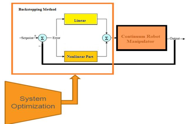
Fig.1: Backstepping Optimization Control Methodology with Application to Continuum Robot [1]
