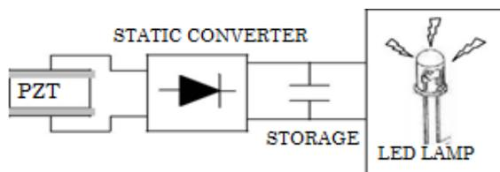
Fig 2: Bike LED lamp supply using piezoelectric material
