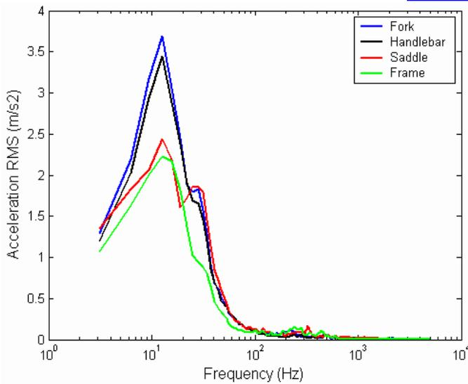
Fig 2: Vibrations acceleration measurement for the case of a bike rolling on uneven path at 8 km/h speed
