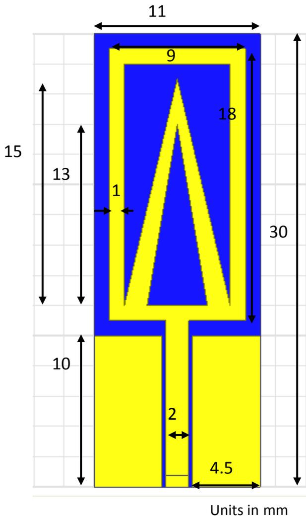
Fig.1. Configuration of proposed compact CPW antenna
