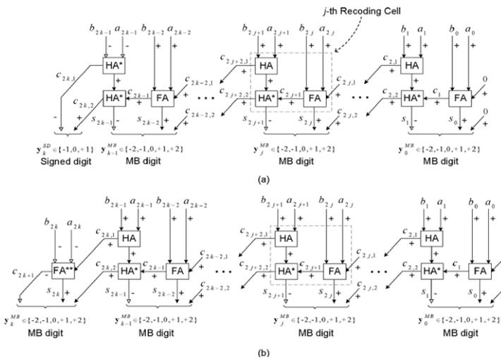
Fig. S-MB2 recoding scheme for a) Even and b) Odd number of bits
