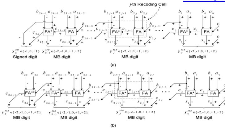
Fig. S-MB1 recoding scheme for a) Even and b) Odd number of bits
