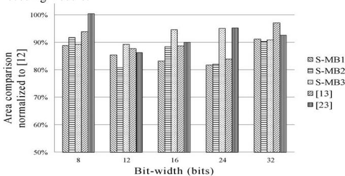
Fig. 4. Area comparison for even bit-width with all values normalized to the corresponding ones of [12].
