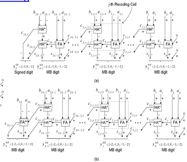
Fig. S-MB3 recoding scheme for a) Even and b) Odd number of bits
