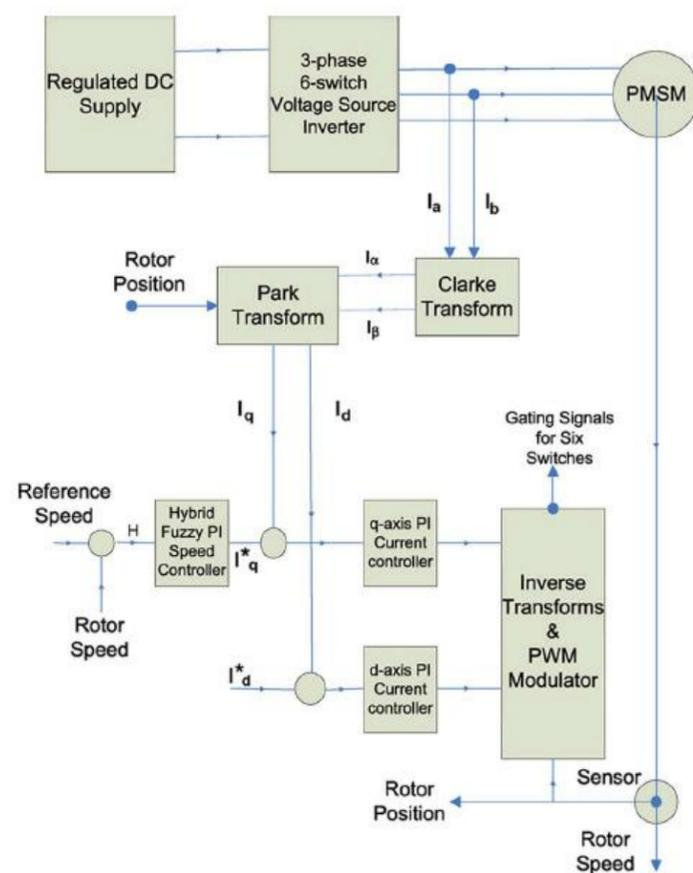
Fig.1. Schematic diagram of the vector control of PMSM with hybrid fuzzy-PI speed controller and PI current controllers.
