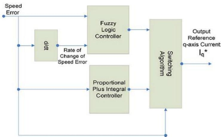
Fig.2. Schematic diagram of hybrid fuzzy-PI controller with switching function.
