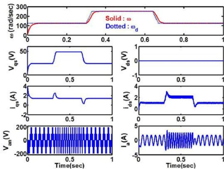
Fig. 4. Simulation results under 200% variations of some parameters ( $R_s$ ,  $L_s$ ,  $J$ ,  $T_L$ , and  $\lambda_m$ ).
