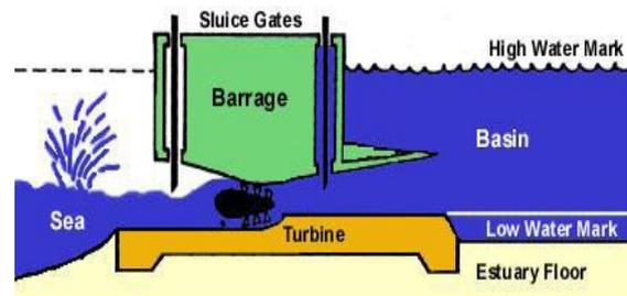
The components of a tidal power station are:
