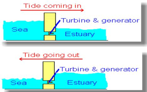
Fig. 3.6.1 - Simple draw of the operating condition of a two-ways barrage tidal power plant (Andy Darvill,
